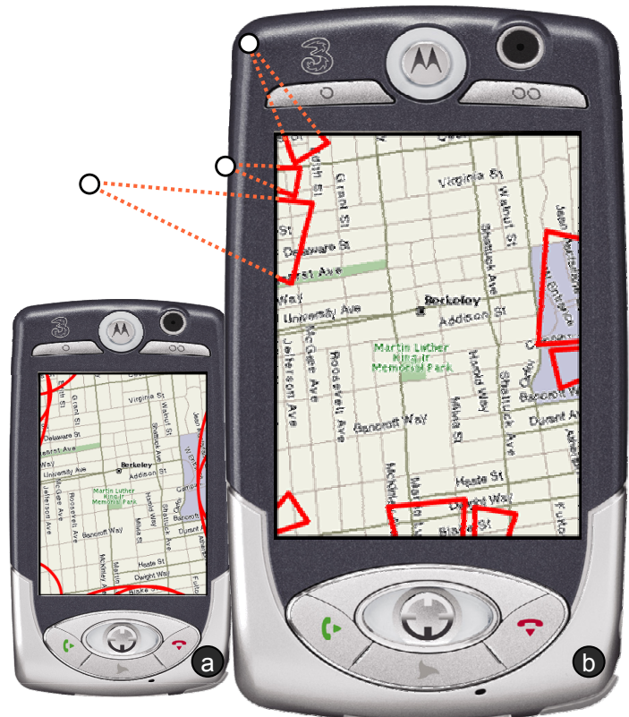
Figure 1: (a) The problem: Halo arcs point users to off-screen targets, but overlapping arcs are hard to interpret. (b) Wedges point to the same off-screen locations; since they avoid overlap, the display remains intelligible.
