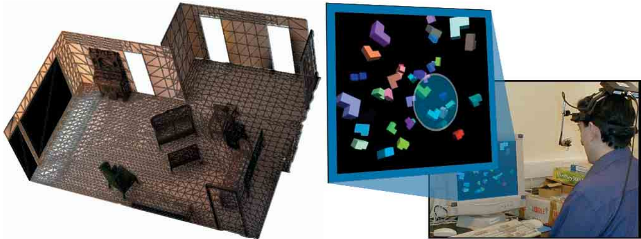
Figure 3. Gaze-contingent spatial and temporal LOD modeling. As the viewer focuses outside the room at the left of the rendering (image at left, courtesy of David Luebke), scene objects located at the right side of the room are rendered using a lower level of spatial detail, indicated by larger triangles (overlaid). Collisions between L-shaped objects (image at right, courtesy of Carol O'Sullivan and John Dingliana) are calculated at a higher level of temporal detail if located within the user's current focus of attention.
