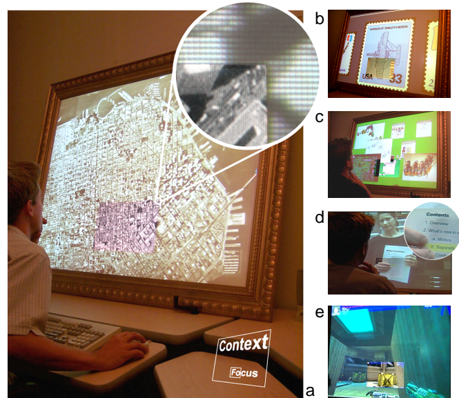
Figure 1: (a) Focus plus context screen prototype. The iconic illustration (bottom right) shows the location of the focus screen. The callout shows the different resolutions of focus and context area. Other application examples (b) Adobe Illustrator (c) Linux desktop (d) videoconferencing and (e) first person shooter game.
